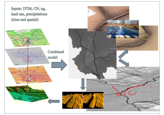
Simplified procedure for the development of the model on the pilot catchment
