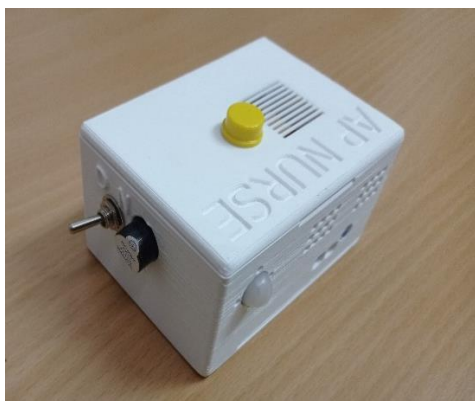
Figure 4. AP4-H device with PIR movement sensor
