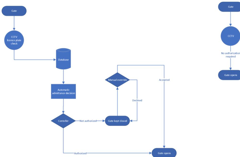
20. Figure - Flowchart of access system of FBL
