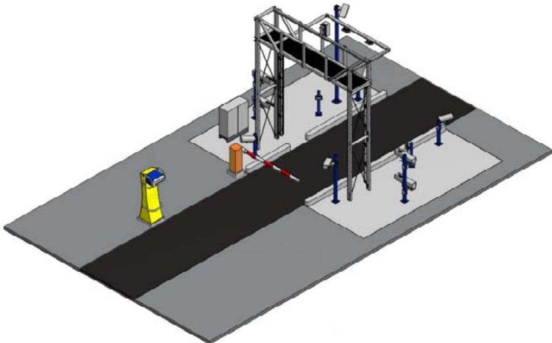
14. Figure - Access control system from CAMCO Technologies (Truck OCR camera portal)
