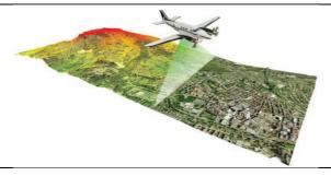
b) aerial 3D survey of the territory which deliver point clouds (LAS format), DTM and DSM
