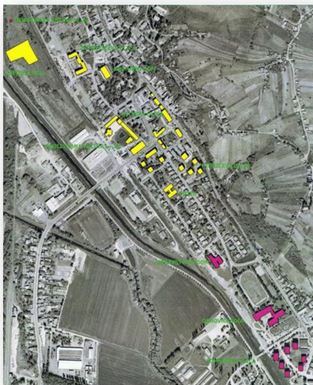
Figure 6: Area of district heating with geothermal energy with all consumers, production and (re)injection well (in yellow - public buildings heated by geothermal energy; in purple - public buildings heated by fossil fuel)
