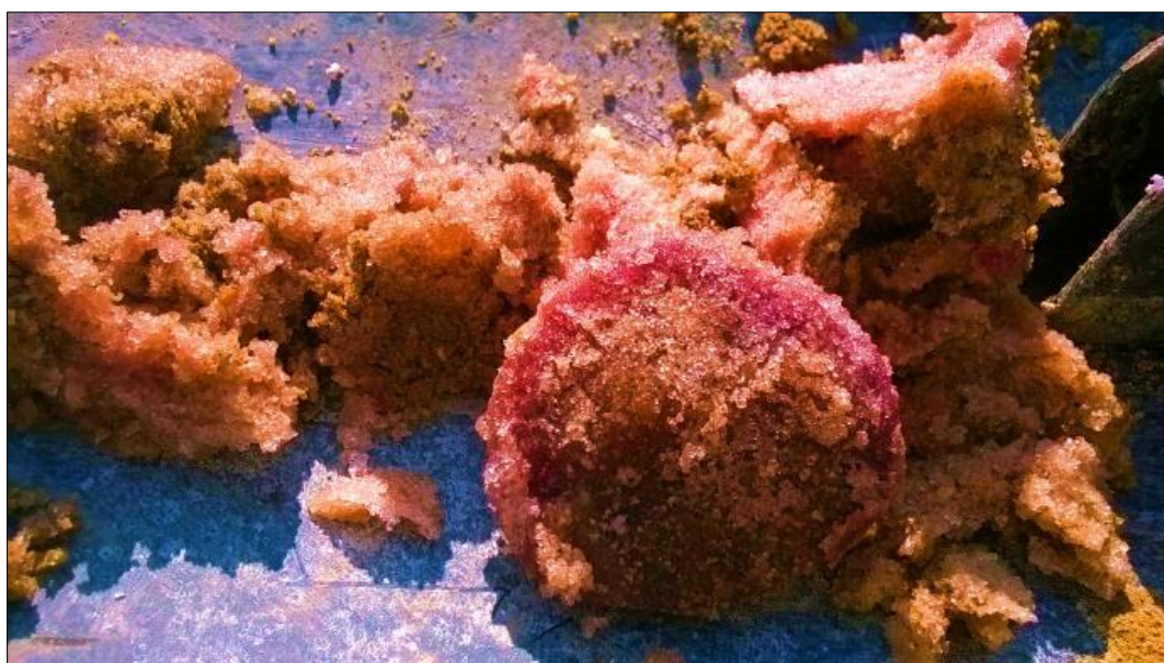
Fig. 17. The recrystallized sodium sulfite heavily contaminated with phenol (by D. Pietrucin)
