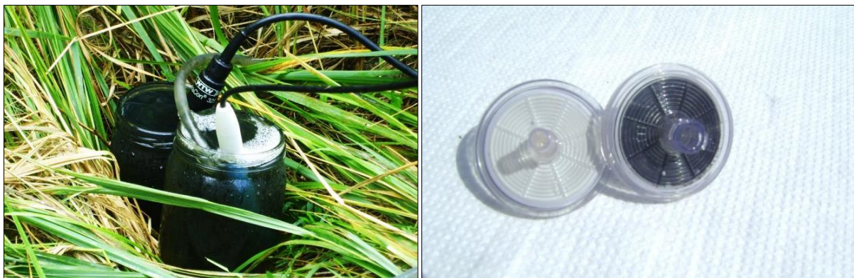
Fig. 14. Heavily contaminated groundwater and a 0.45 µm filter before and after filtration of water (by D. Pietrucin)
