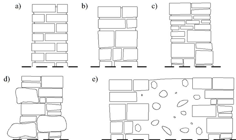
Fig. 1. Selected types of the masonry walls in the ruins of castles - a) wall made of ceramic bricks, b) wall made of stone blocks, c) wall made of stone blocks with leveling layers, c) wall made of broken stones with boulders, d) the „opus emplectum” wall[1]
