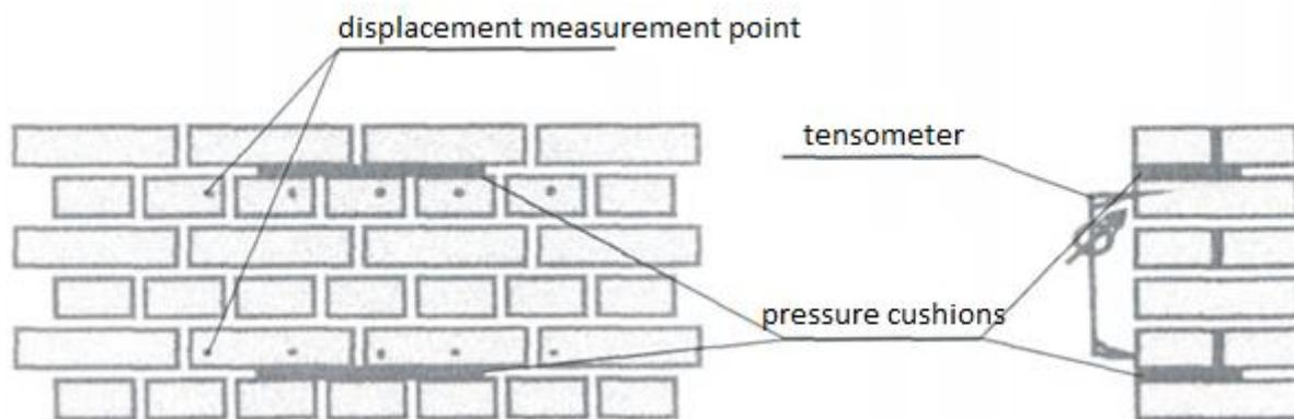
In order to obtain the result of the compressive strength of the wall, it is necessary to put pressure in the cushions to cause local destruction of the masonry structure. The destructive pressure will be the limit strength of the masonry structure. Destruction is not reversible, and the test becomes a destructive test.
