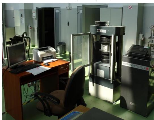
Photo 8 Test stands - the Controls Advantest 9 hydraulic press
