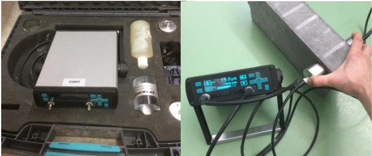
Photo 4 Ultrasonic testing equipment
