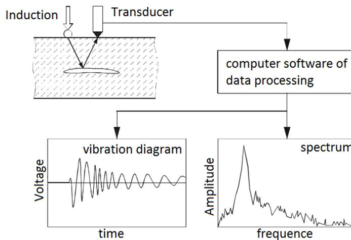
Fig. 6 Scheme of the test 0
