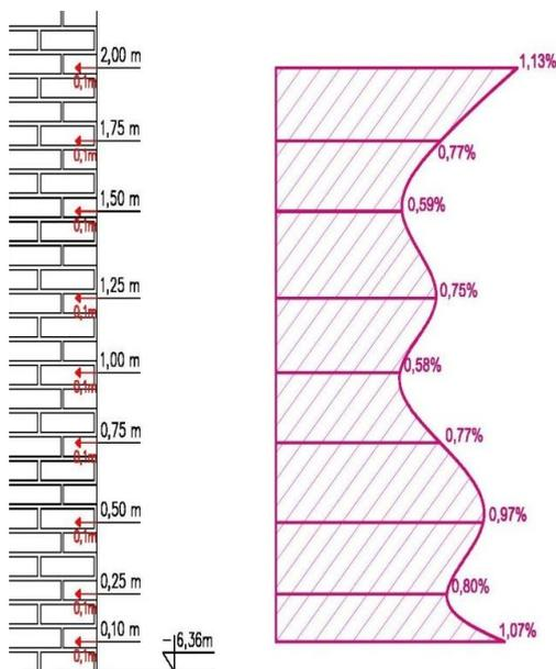
Fig. 16 Diagram of the distribution of salinity with sulphates at the level of the cellar wall at the sampling from the depth of 0.1 m.
