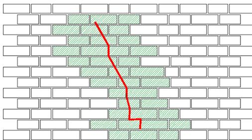
Fig. 7. Scheme of the wall rebuilding
