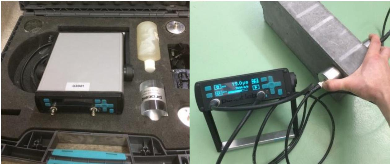
Photo 4 Ultrasonic testing equipment
