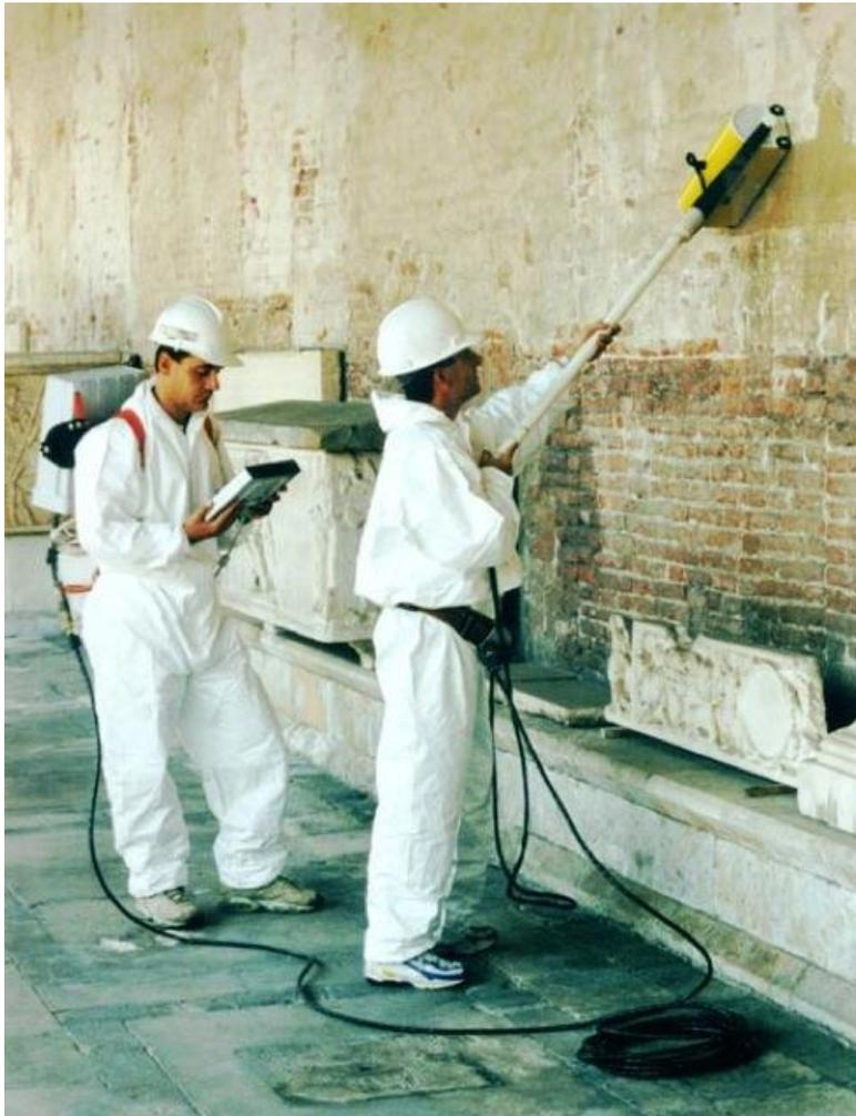
Picture 4: geoelectric prospecting
