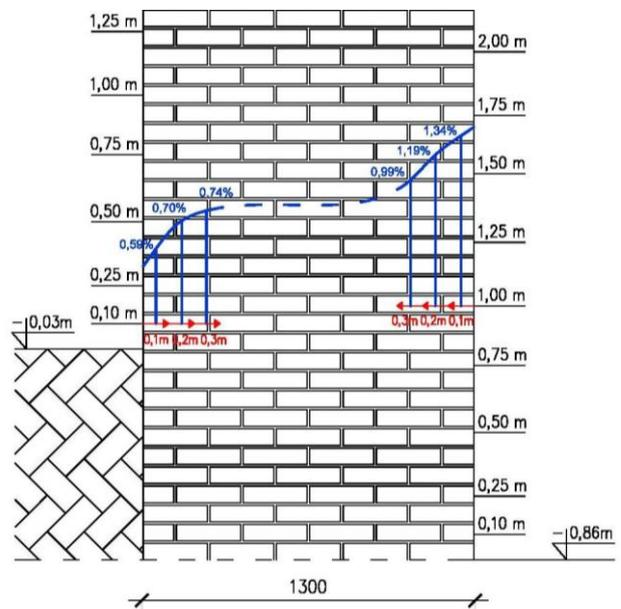
Fig. 17 Diagram of the distribution of salinity with sulphates of the external construction wall at the height of 0.1 m above the ground level.
