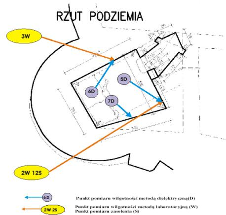
Fig. 15 Sampling points for testing in the basement of the defensive tower of the Janowiec castle
