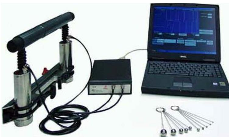
Fig. 7 Hammer test set (source: <http://www.impact-echo.com/Impact-Echo/images/wssetup.jpg>)
