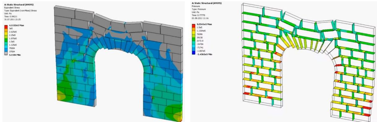
Fig. 18 View of stresses in a wall element and joints (source: <https://i.ytimg.com/vi/sMpNE9L2reY/maxresdefault.jpg>)
