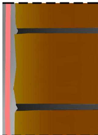
Fig. 12 Salt corrosion inside the plaster layer
