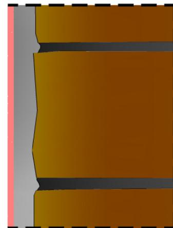
Fig. 13 Salt corrosion on the surface of the plaster
