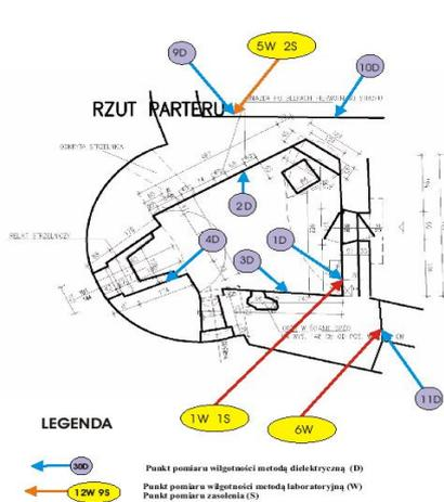
Fig. 14 Sampling points for tests on the ground floor of the defensive tower of the Janowiec castle
