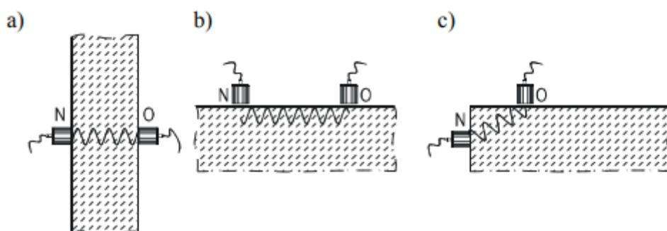
Fig. 5 Scheme of measurements performing and distribution of probes
