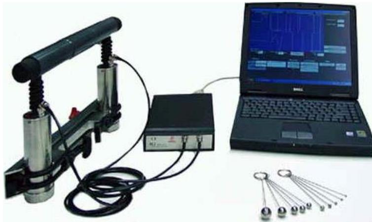
Fig. 7 Hammer test set (source: <http://www.impact-echo.com/Impact-Echo/images/wssetup.jpg>)
