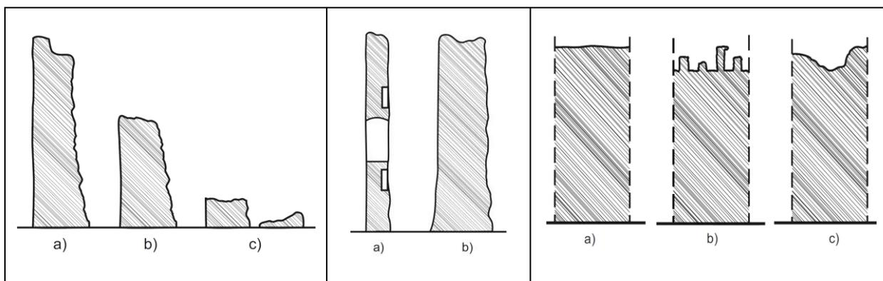
Fig. 1 The division of walls with respect to height: a) a high wall, b) a medium wall, c) a low wall
