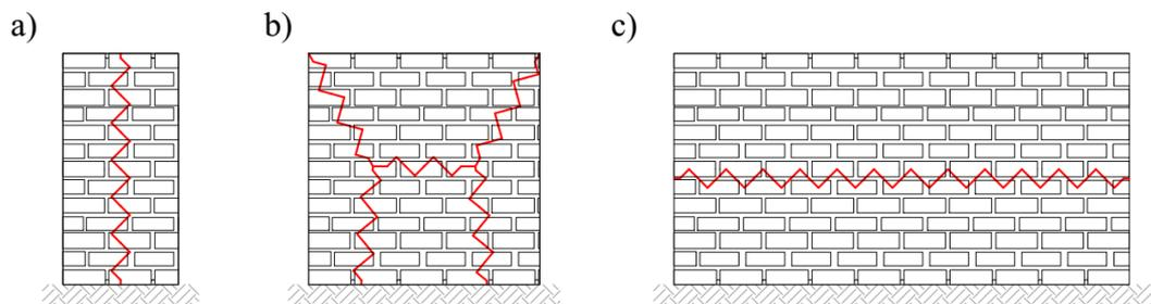
Fig. 5. Damage to the brick elements caused by excessive horizontal force (perpendicular to the element's plane) depending on the proportion of the element: a) slender elements, b) similar height and length, c) elements with a significant length in relation to the height [2].
