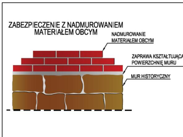
Fig. 20 Addition made of foreign material / A securing layer - addition of a foreign material/ Addition of a foreign material/ Mortar giving shape to the wall surface/ The historic wall
