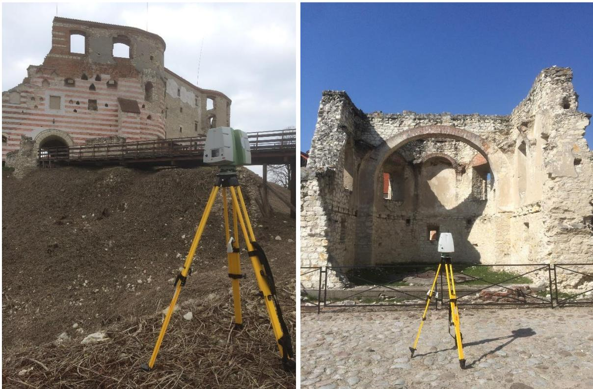
Photo 3 The Leica C10 scanner during field work at the Castle in Janowiec.
