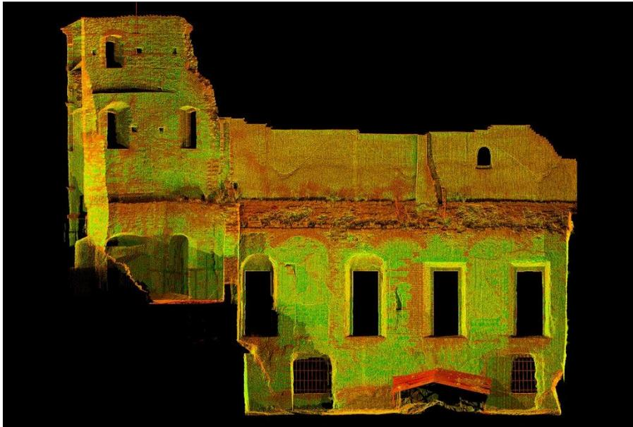
Fig. 2 Image of the southern wall of the courtyard obtained from the cloud of points.
