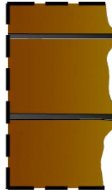
Fig. 10 Salt corrosion of the wall surface with mortar stronger than the masonry material.
