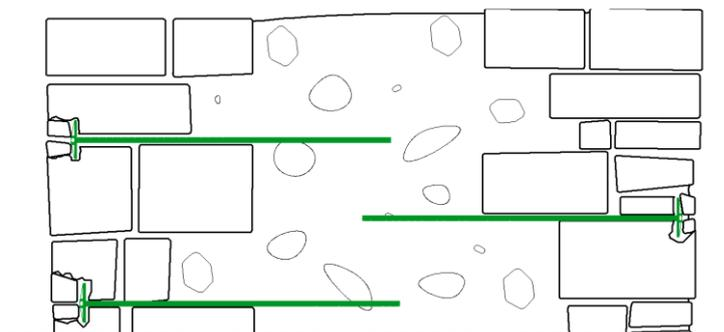
Fig. 9. Scheme of nailing with the supplementation of the wall's face of the „opus emplectum” type
