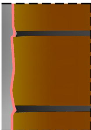
Fig. 11 Salt corrosion at the interface between plaster and masonry
