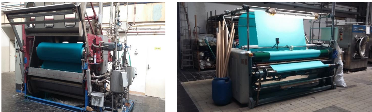
Fig. 5: Dyeing and measuring of the fabric with photocatalytic phtalocyanine dyestuffs
