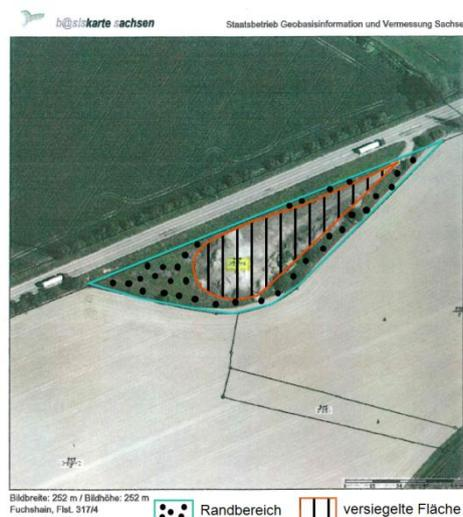
Figure 2. Site plan for the property in Naunhof/Fuchshain (in red are the existing sealed areas, in blue are the surrounding areas)
