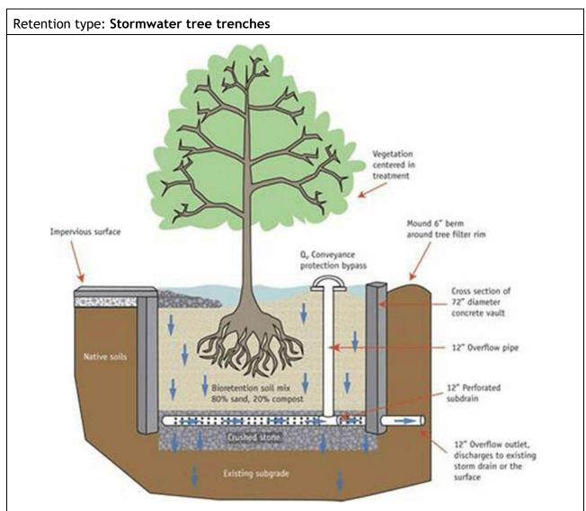
Figure: 39. Stormwater tree trench (https://mediaborough.blog/2018/05/17/stormwater-projects-in-the-borough/#jp-carousel-108)
