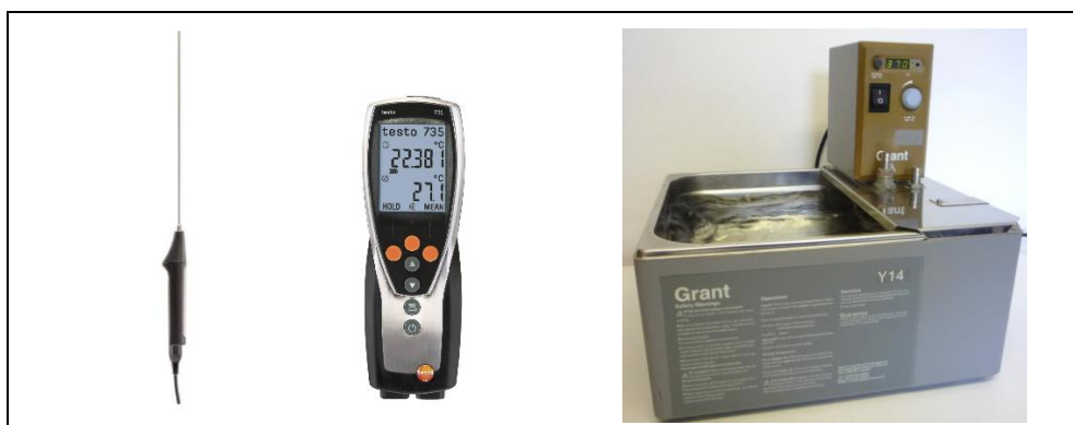
Figure 2: calibration equipment: testo reference sensor with handheld device (left); Grant temperature regulated water bath (right), source: testo.com, labmerchant.com
