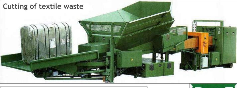
Cutting line "ROBOT" - Up to 8000 kg/h
