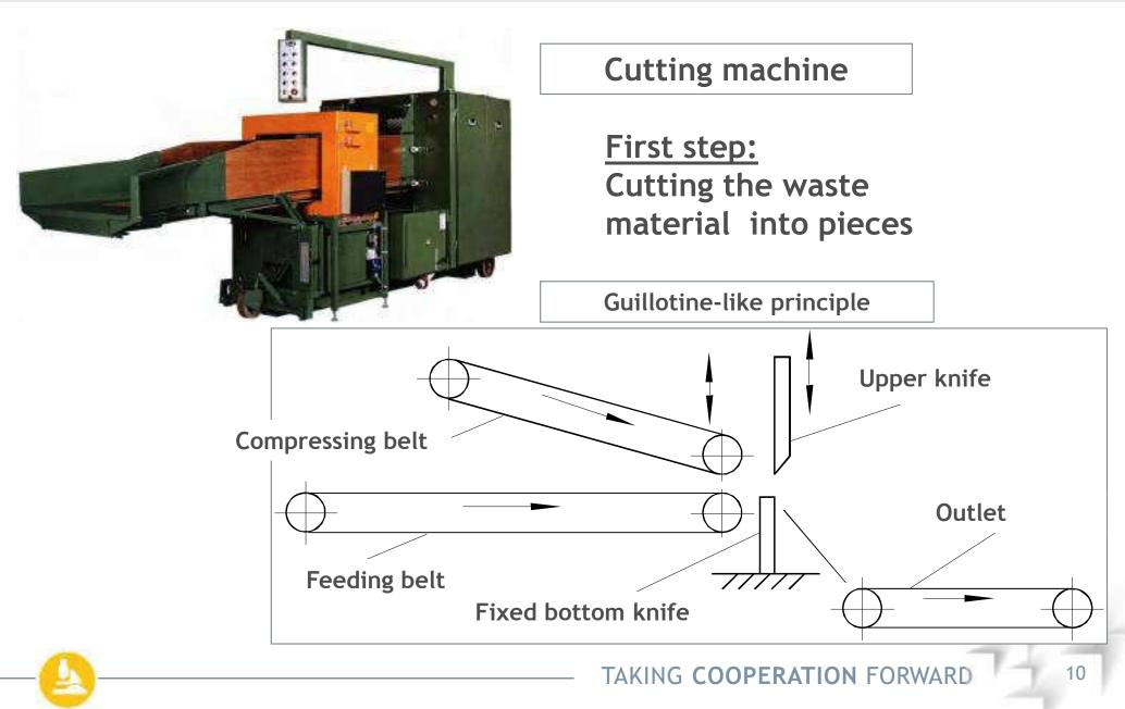
PROCESSING OF TEXTILE WASTE -TEARING PROCESS PRINCIPLE
