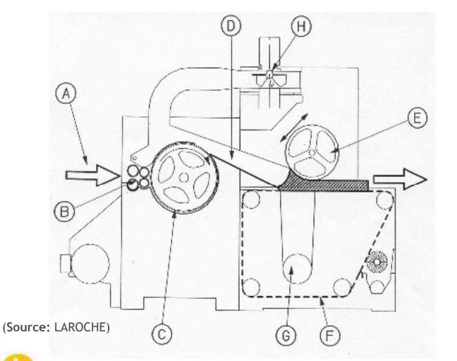
A Fibre fluff B Material feed C Opening roller D Air channel E Pressure roller F Sieving conveyor G Intake suction H Additional air
