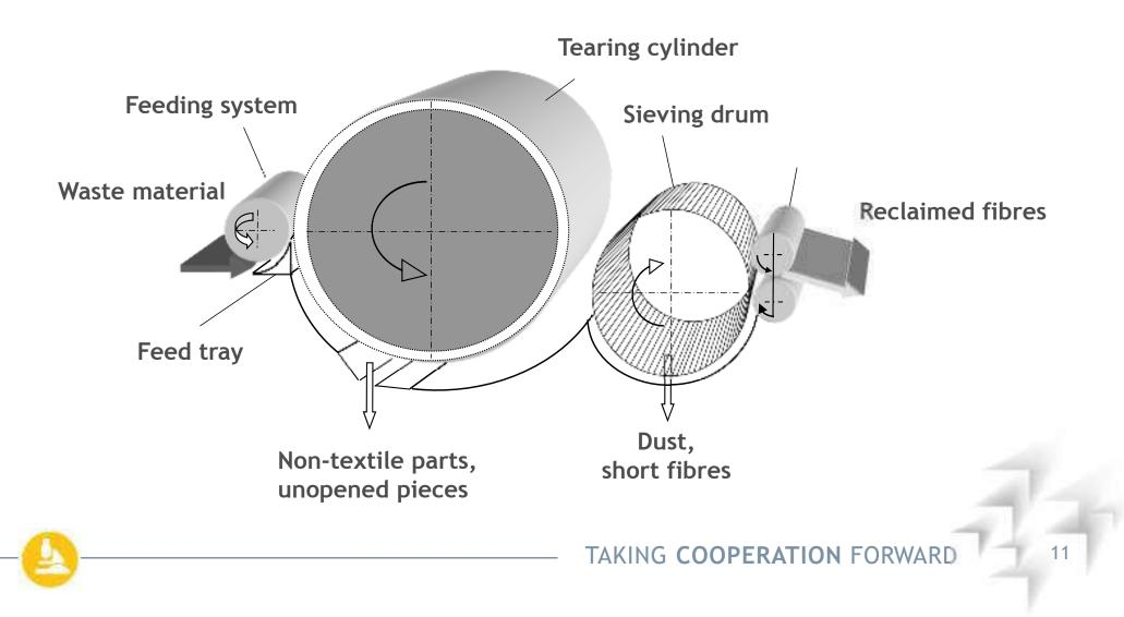
PROCESSING OF TEXTILE WASTE -TEARING PROCESS PRINCIPLE
