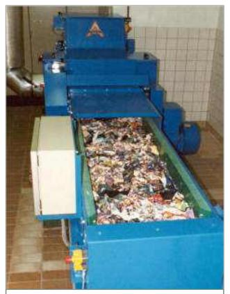
Lab-scale tearing machine
