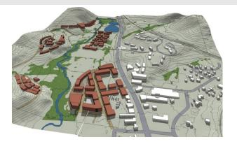
**3D data model** use a combination of geometric primitives to represent reality with 3D object. Attributes include positions, shape and size, beside textual and numerical information.
