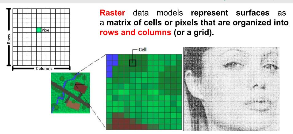
Each cell/pixel **contains a value representing dat**a (e.g. information such as temperature, height, PV potential, etc.). **Raster's are:** orthophotos, satellite imagery or even scanned maps.
