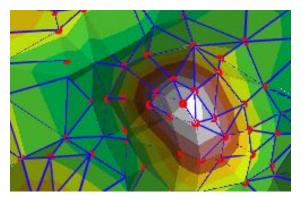
**TIN** (*Triangulated Irregular Network*) is a network of triangles connected together to create a 2.5D surface where the triangles in this network are not crossing.
