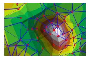
**TIN** (*Triangulated Irregular Network*) is a network of triangles connected together to create a 2.5D surface where the triangles in this network are not crossing.
