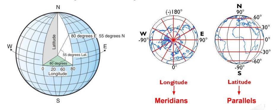
Among the most used GCS, we have the **WGS84** (World Geodetic Survey 1984), also used for GPS measurements.
