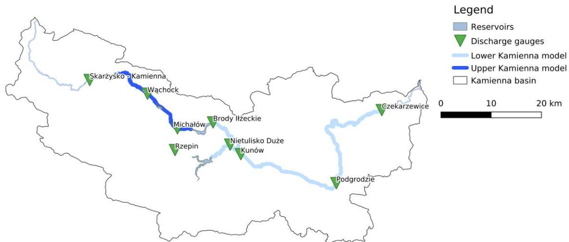
Figure 19: Model structure - division between Lower and Upper Kamienna models
