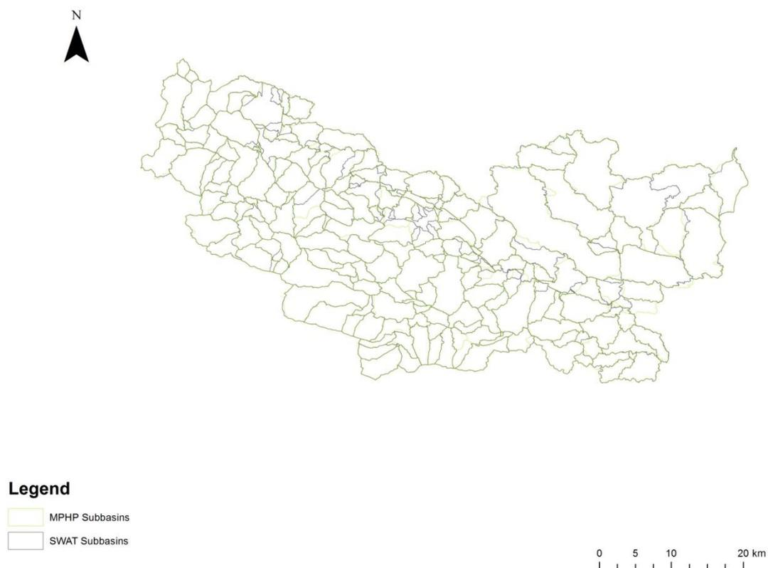
Figure 3 – Subcatchments subdivision of the delineated watershed compared to real subbasin division (MPHP – official hydrography map).
