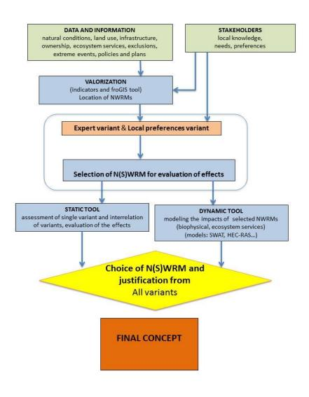
Figure 1. Main steps of the concept plan elaboration
