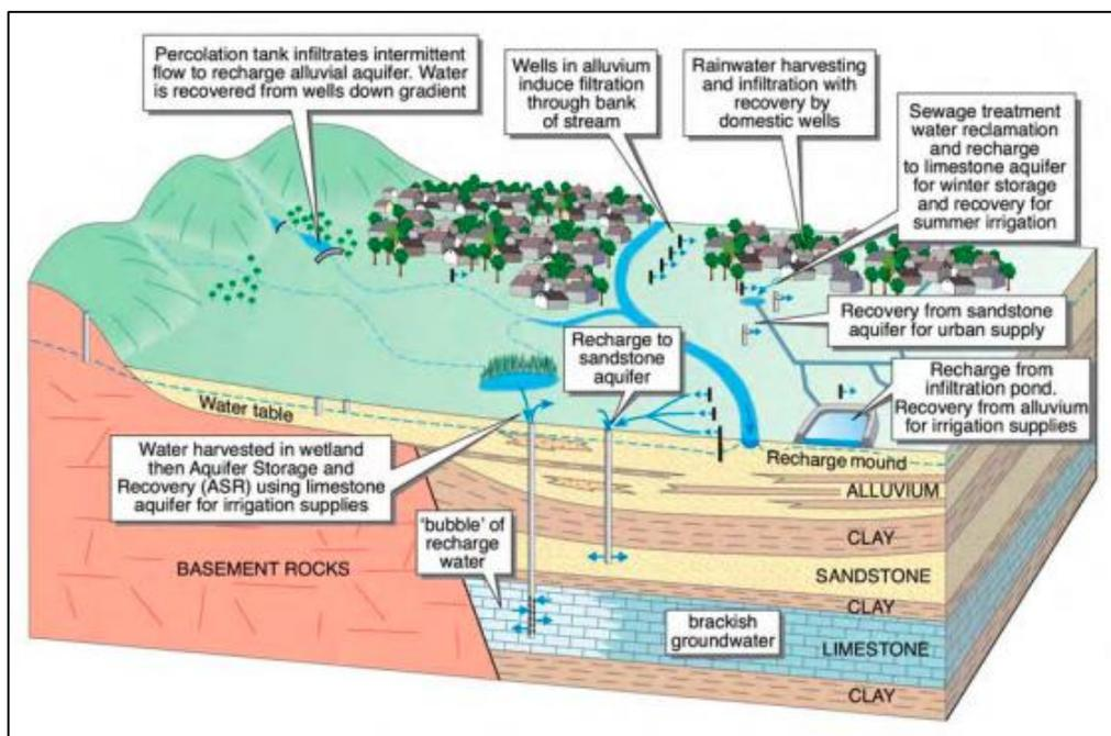
**Figure 1:** Illustration of MAR applications as a function of geographical, geological and hydrogeological conditions (Dillon et al., 2009)
