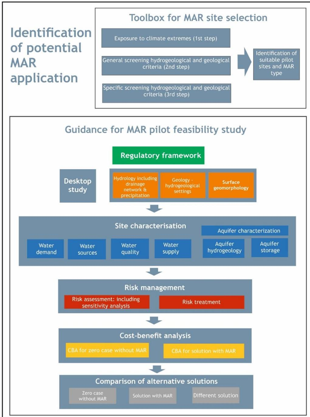
**Figure 2:** Procedure for the identification of potential MAR application, implementing the decision support toolbox for MAR site selection (on top) and the common methodological guidance for MAR pilot feasibility studies (bottom) (DEEPWATER-CE(2020b))
