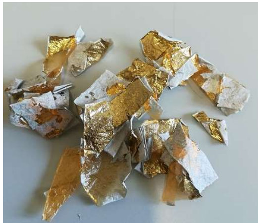
Solid board: paper laminated with metalized PET film
