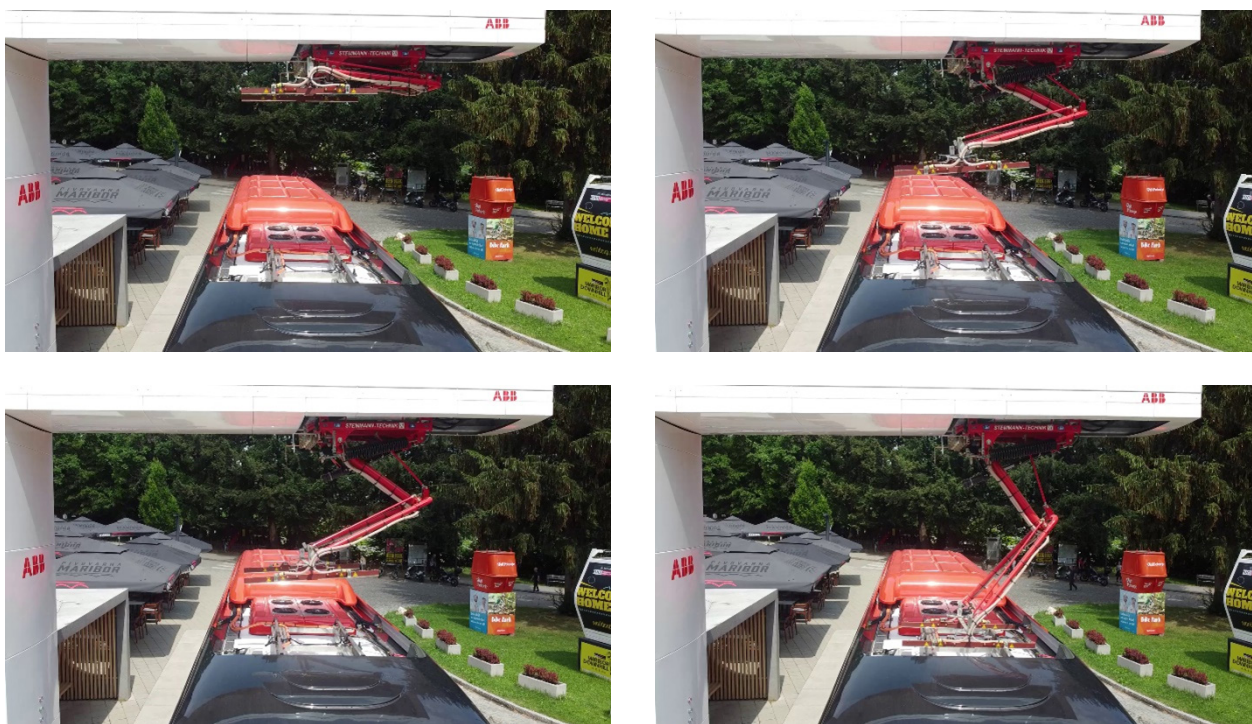
Figure 22: Demonstration of the operation of the pantograph
