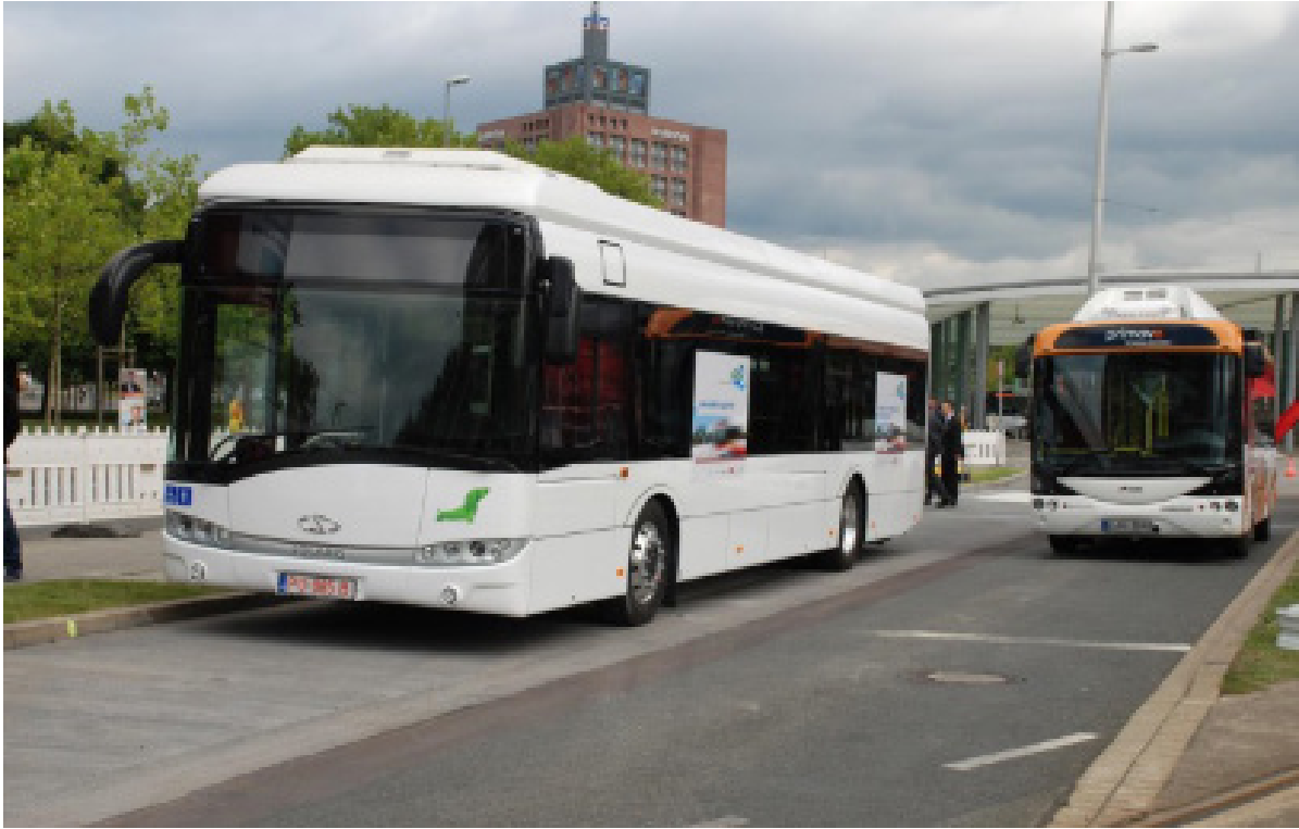
Figure 15: E-bus with inductive charging in Braunschweig. Source: Rupprecht Consult.
