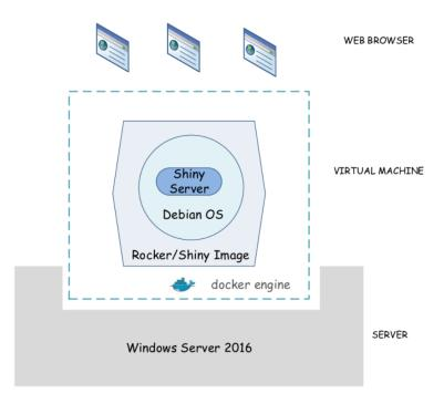
Fig. 1 Structure of the GIS Tools application
