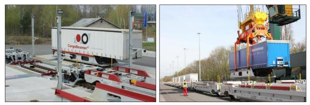
Figure 9: system CargoBeamer<sup>2</sup>: horizontal (left) and vertical (right) handling
