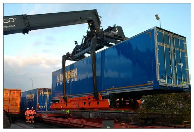
Figure 7: Loading system VEGA (source: www.roadraillink.eu)
