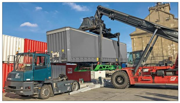
Figure 6: Loading system NiKRASA in the MAHART intermodal terminal in Budapest (source: www.dvz.de)
