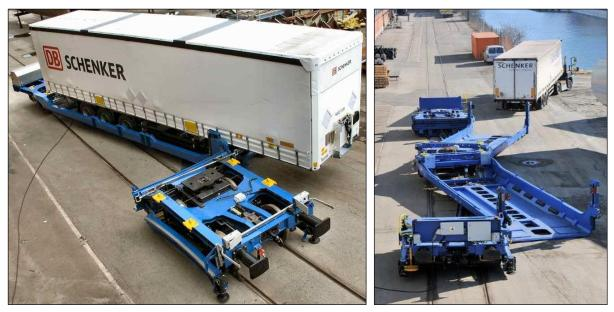
Figure 14: system Megaswing: loading process
