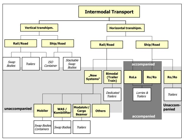
Figure 3: Intermodal handling technologies
