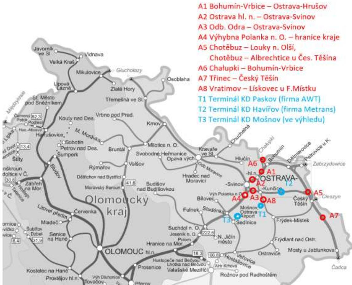
The map above shows the individual bottlenecks on the SŽDC network. The most restrictive sections on the SŽDC network are points A1 and A2. At points T1, T2 the significant terminals KD are shown. The terminal in Mošnov (point T3) will be built in view.
