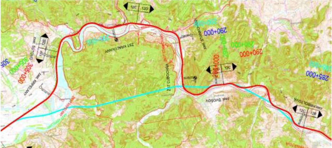
The blue route represents the solution with the highest line speed and the greatest time savings, the disadvantage of this solution is the necessity to build several tunnels, where the longest tunnel is more than 7 km long. The red variant copies the current trace.
