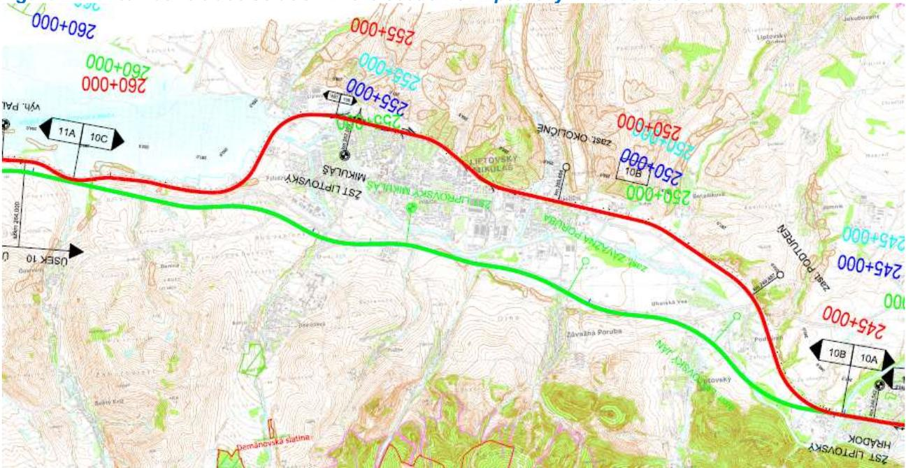
The proposed solution marked in green line, which will bring the highest line speed and at the same time the greatest shortening of the travel distance. This option proposes to move the railway station Liptovský Mikuláš out of the city center. The red line indicates the current route guidance in this section.
