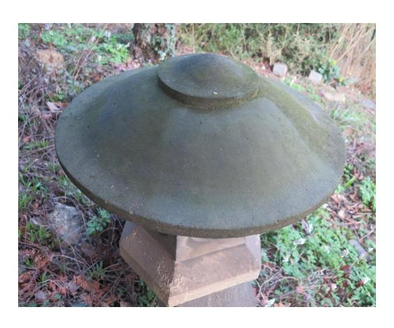
Test of function of photoactive coating on sandstone lantern, which become green because of algae deposition—part of lantern is coated, photo taken after 2 months
